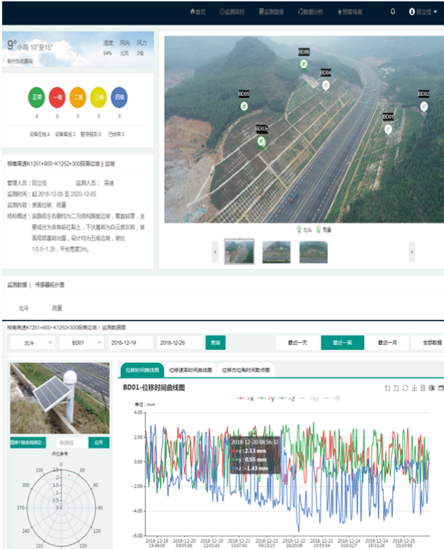
Fig. 2. BDS monitoring system platform and monitoring data display
