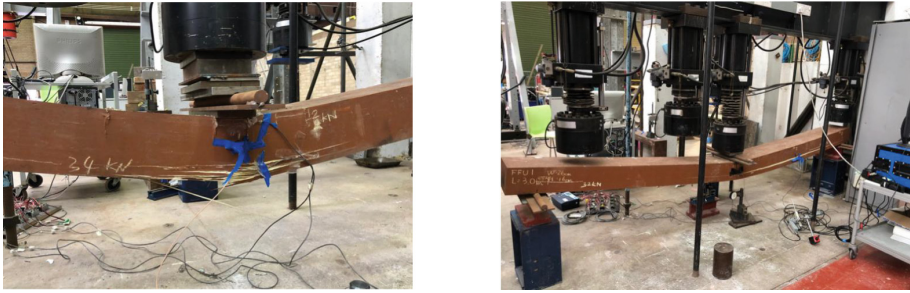
Fig. 8. Failure mode of full-scale FFU composite beams under flexural load [28].
